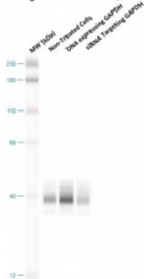
Figure 6. Protein expression of GAPDH in MCF-7 cells. DNA plasmid expressing GAPDH or siRNA targeting GAPDH were transfected into MCF-7 cells following Altogen Biosystems transfection protocol. At 72 hours post-transfection the cells were analyzed by Western Blot for protein expression levels (normalized by total protein, 10 \mu g of total protein loaded per each well). Untreated cells used as a negative control.
